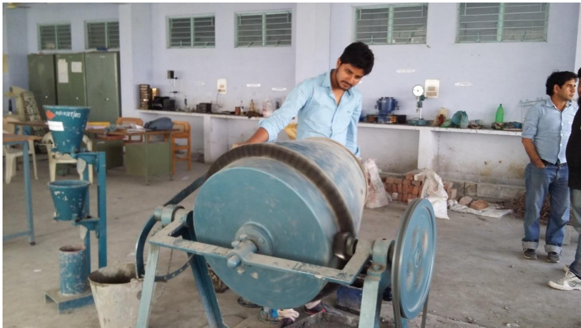
Mixing of Concrete by Mechanical Mixer
